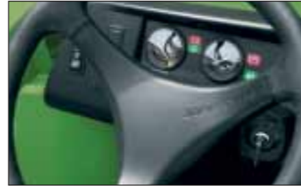
Gauge Package Electronic speedometer and voltmeter analogue gauges integrated in the instrument panel. Good for precision tasks. T
