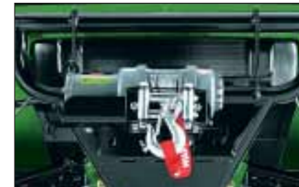
Winch Warn® Winch has rated line pull of. 1134 kg. Move logs, pull out bushes with control or tension fences. Quiet, three-stage planetary gear design offers increased efficiency and improved load distribution. T HP XUV
