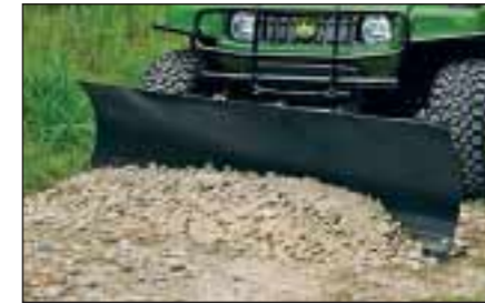
Blade 1.83 m (72 in) Light duty, three-position blade comes with a standard power lift and two adjustable skid shoes. Attaches quickly with two pins and one link. T HP XUV
