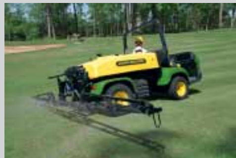
Spray it down. The HD200 Sprayer features a 750-litre capacity tank and rugged multi purpose 5486 mm booms range from 4.6 – 6.4 metres.
