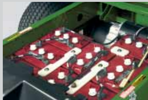
The TE Gator batteries , which use a 48-volt system, have more lead than typical electric utility vehicles, so they hold their charge longer.
