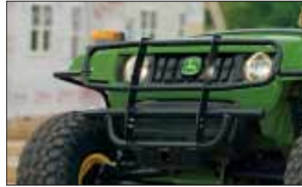
Brush Guard Strong bumper-mounted guard shields headlights. T
