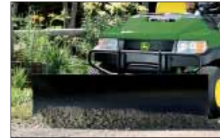
Blade 1.37 m (54 in) Light-duty three-position blade has a replaceable cutting edge and two adjustable skid shoes. Separately sold Quick-Attach system allows drive up attachment. Optional plough markers enable operator to easily see blade edges. C
