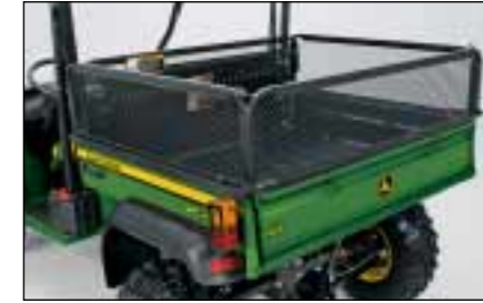
Cargo Box Side Extension Four-sided structure that increases cargo box side height to 533 mm and volume to 0.74 m 3 . T* HP XUV *not for TS
